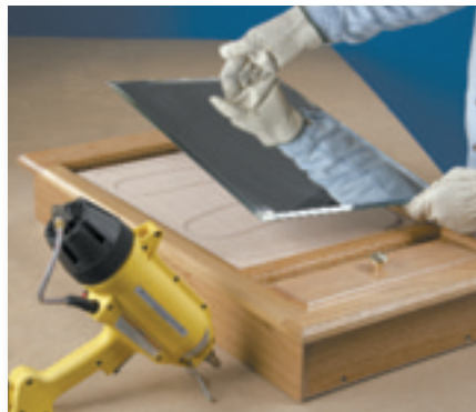
Long open time provides production speed flexibility for bonding a mirror to plywood or MDF panel in a medicine cabinet door.
