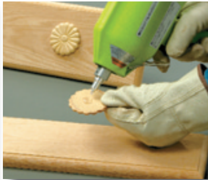
17 Bond wood or plastic rosettes to wood drawers without fixturing or drying time.
